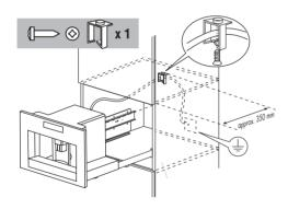
Fix the power cable with the clip.
