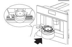
The coffee spout (A13) must be fully raised to enable the jug to be inserted.
