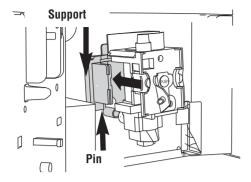
**N.B.!** If the brewing unit is difficult to insert, you must first adapt it to the right dimensions by pressing it forcefully from the bottom and top as shown in the figure.
