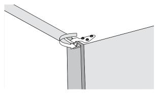
Loosening the top hinge fasteners will allow the top hinge to be slightly rotated thus adjusting the gap between doors.
