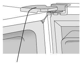
Small plastic clip is located here. With the door open, pull the cover outward while simultaneously pulling up in order to release the hinge cover.
