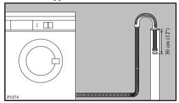
The standpipe should have an internal diameter of approximately 38mm (see diagram) thus ensuring there is an air break between the drain hose and standpipe.
