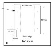
Fix the base firmly to the floor using four appropriate countersunk screws (see Fig. H).
