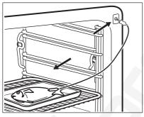
Insert the tip of the Food Sensor exactly in the centre of the casserole. The Food Sensor should be stabilized in one place during baking. Use a solid ingredient to achieve that. Use the rim of the baking dish to support the silicone handle of the Food Sensor. The tip of the Food Sensor should not touch the bottom of a baking dish. Cover the Food Sensor with the remaining ingredients.
