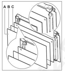
Make sure that you put the glass panels (C, B and A) back in the correct sequence. First, insert panel C, which has a square printed on the left side and a triangle on the right side. You will also find those symbols embossed on the door frame. The triangle symbol on the glass must match the triangle on the door frame, and the square symbol must match the square. After that insert the other two glass panels.
