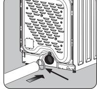
2. Carefully slide the dryer to its final position. Adjust one or more of the legs until the dryer is resting solidly on all four legs. Place a level on top of the dryer. The dryer MUST be level and resting solidly on all four legs. Rock alternating corners to check for stability.
