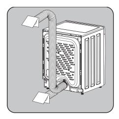
If installing flexible metal (semi-rigid) venting, do not exceed 2 m total duct length.
