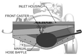
**2C. ONBOARD HOSE BAFFLE:** If your machine is equipped with the optional **Onboard Hose Baffle**, simply press down on the **Baffle Control Handle** to release the locking pin and rotate it clockwise as far as it will go.
