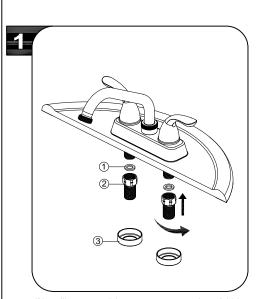
If installing onto a sink or countertop more than 1" thick, from underside, assemble washer (1), connector (2) and mounting bracket (3) onto body. NOTE: If installing onto a sink or countertop more than 2" thick. Mounting bracket (3) should be discarded.
