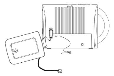
3.) Adjust the angle of the loop antenna until you find the position that provides the best AM reception.
