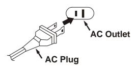
make the plug fit into your outlet. This defeats the safety feature and could expose you to electric shock.
