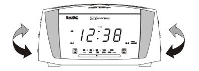
**FM** – The FM antenna is built in to the Mains power cord. If FM reception is weak try varying the position and direction of the power cord until you find the strongest signal.
