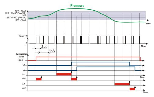
The capacity of the DGS compressor is limited by the PM and PMA parameters, where
