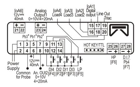
Power supply: model at 12Vac/dc supply: use terminals 1-2 Power supply: model at 124Vac/dc supply: use terminals 1-2
