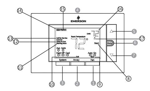
Whenever "Feplace" appears in the display, new premium brand AA alkaline batteries should be installed. If the house will be unoccupied for an extended period and either "Feplace" is displayed, install new batteries before leaving.
