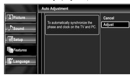
The horizontal/vertical position, clock and phase of the PC screen are automatically adjusted.
