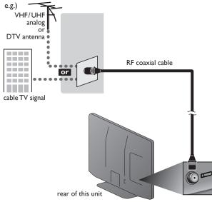
Once connections are completed, turn on the unit and begin initial setup. Channel scanning is necessary for the unit to memorize all
