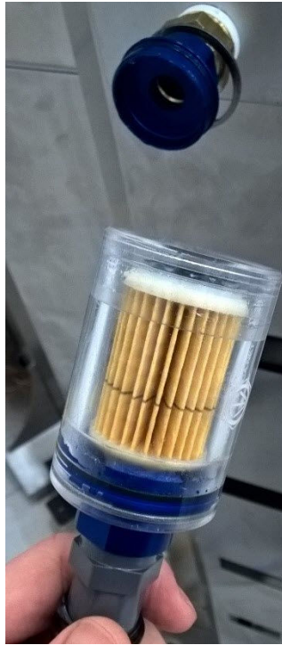
Figure 7-5: Removing the End Fitting from the Filter Housing
