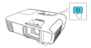
**Note:** To shut down the projector, press the  $\bigcirc$  power button twice.
