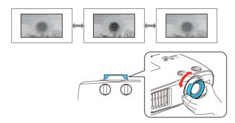
If your image is uneven on the sides, you can use the keystone correction feature to adjust the image. To use this feature, you must first set the lens to the center-top position using the lens shift dials.
