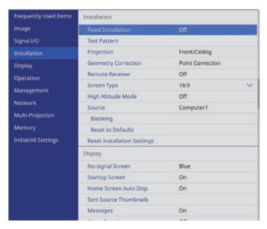
Select **Geometry Correction** and press [Enter]. The **Geometry Correction** screen is displayed.
