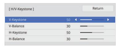
Use the arrow buttons on the projector or the remote control to select between vertical and horizontal keystone correction and to adjust the image shape as necessary.
