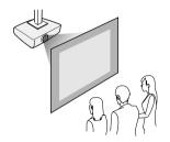
Select the correct **Projection** option in the projector's **Installation** menu according to the installation method being used. If necessary, turn on the **Inv Direction Button** setting in the projector's **Operation** menu and adjust the **Menu Rotation** setting in the projector's **Display** menu.
