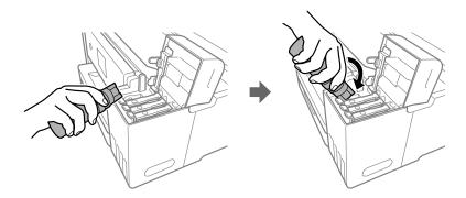
**Note:** Refer to the color-coded sticker on the ink tank unit to identify the color of each tank. Do not force the bottles into position; they are keyed for each color.
