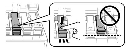
**Note:** If any ink remains in the bottle, replace the bottle cap and tighten it. Store the bottle upright for later use.
