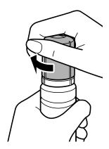
**Caution:** Do not shake or squeeze the bottle. Do not touch the top of the bottle after its cap is removed.
