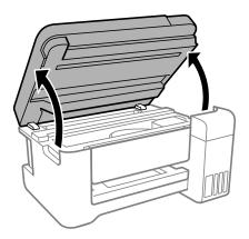
3. Open the ink tank cover, then open the cap for the ink tank you are going to fill.
