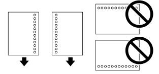
• To load a sheet of paper longer than legal size, close the paper support and output tray, then flatten the leading edge of the paper as shown.
