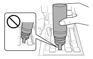
**Note:** If ink does not flow from the bottle, lift and reinsert the bottle.
