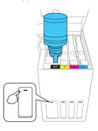
**Note:** If ink does not flow from the bottle, lift and reinsert the bottle.
