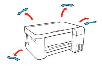
**2** Lift up the scanner unit. Remove all protective materials from inside the product.
