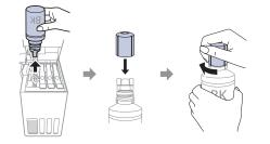
**Note:** Do not leave the ink bottle inserted; otherwise the bottle may be damaged or ink may leak.
