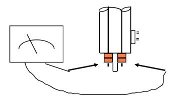
If the reading is less than 20 ohms on the "Rx 1" scale or the "Rx 10" scale the element is good, if it is much greater e.g.... 10,000 ohms or if you get a reading on the "Rx 1K" scale then you must replace the element (contact Eemax). Tel: 1-800-543-6163 for replacement elements.
