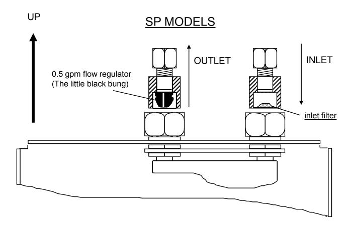
If the heater now turns "on" with water flowing, call Eemax at 1-800-543-6163. Describe what you have done and we will send you a selection of "bungs" to replace the one which you have removed. This will allow the unit to turn "on" but will also control the flow rate to give you the correct rise in temperature.
