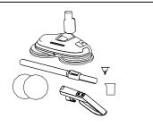
Slide the bottom end of Telescopic pipe onto the polisher head until pipe button clicks into place.
