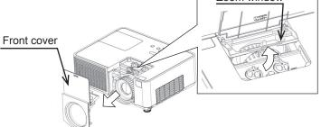
2.Insert your finger from the side, turn the lens to the left and remove while pulling up on the lens lock lever, as shown in the illustration.
