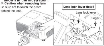
3.Attach the replacement projection lens.
