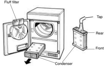
**Every Month** Remove condenser unit and clean any build up of fluff from between the plates by rinsing it under the tap with cold water. This should be done with cold water from the rear of the condenser. Refit with the handle at the front.
