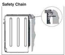
! In order to prevent accidental tipping of the appliance, for example by a child climbing onto the oven door, the supplied safety chain MUST be installed!
