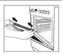
5.Remove the glass sheet and do the cleaning as indicated in chapter: "Care and maintenance".
