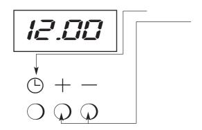
Step 3 Press the "L" button and then press either the "+" or "-" buttons to set the correct time of day.
