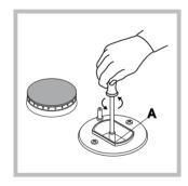
On completing the operation, replace the old rating label with the one showing the new type of gas; the sticker is available from our Service Centres.
