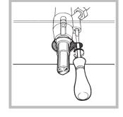
N.B.: In the case of liquid gas, the regulation screw must be screwed in all the way.
