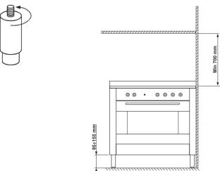
In the lower part of the cooker there are 4 height adjustable screw-in feet with which it is possible to level the cooker if necessary.
