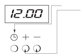
Step 3 Press the " button and then press either the "+" or "-" buttons to set the correct time of day.
