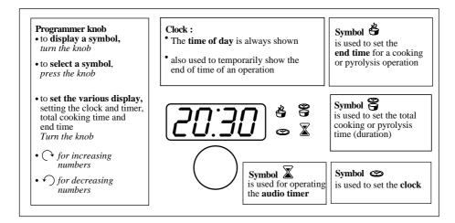
The "24 hour" electronic programmer enables the user to set the duration and end time of a cooking operation for any time within the upcoming 24 hours.
