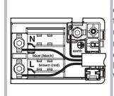
3. Remove the wire contact screws L-N-++, then fasten the wires under the screw heads, respecting the colour code: Black/Blue (N), Red/Brown (L) and Bare Wire/Yellow-Green (++).
