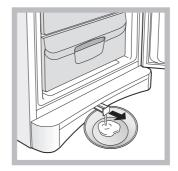
5. Certain appliances are fitted with the DRAIN SYSTEM to lead the water outside. Let the water flow into a container (see diagram).
