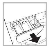
Remove the dispenser by raising it and pulling it out (see figure). Wash it under running wa-
