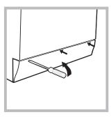
3. using a screwdriver, remove the cover panel on the lower front part of the Washer-dryer (*see figure*).
