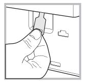
5. reposition the panel, making sure the hooks are securely in place before you push it onto the appliance.
