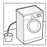
1. remove the plug from the electrical socket. 2. make sure the water level inside the machine is lower than the door opening; if it is not, remove excess water using the drain hose, collecting it in a bucket as indicated in the
