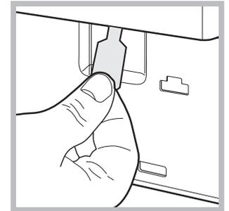
4. Pull outwards using the tab as indicated in the figure, until the plastic tie-rod is freed from its stop position; pull downwards and open the door at the same time.
