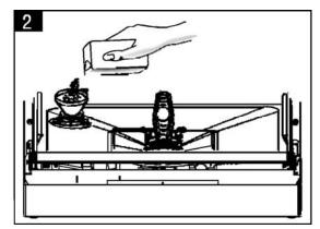
Remove the basket and then unscrew and remove the cap from the salt container.
