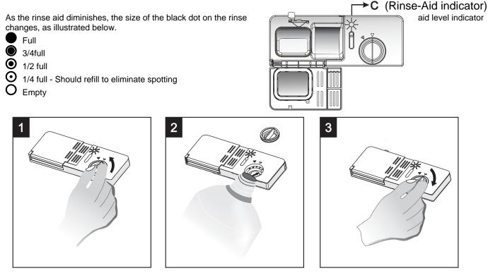
To open the dispenser, turn the cap to the "open" (left) arrow and lift it out.
