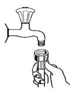
Connect the cold water supply hose to a threaded 3/4 (inch) connector and make sure that it is fastened tightly in place. If the water pipes are new or have not been used for an extended period of time, let the water run to make sure that the water is clear and free of impurities. If this precaution is not taken, there is a risk that the water inlet can get blocked and damage the appliance.
