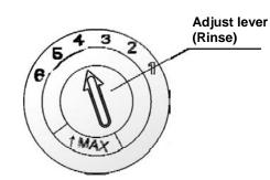
The rinse aid dispenser has six or four settings. Always start with the dispenser set on "4". If spots and poor drying are problems, increase the amount of rinse aid dispensed by removing the dispenser lid and rotating the dial to "5". If the dishes still are not drying properly or are spotted, adjust the dial to the next higher number until your dishes are spot-free. The recommended setting is "4". (Factory value is "4".)
