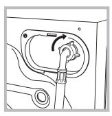
2. Connect the other end of the water inlet hose to the washing machine, screwing it onto the appliance's cold water inlet, situated on the top right-hand side on the rear of the appliance (see figure).
