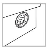
2. unscrew the lid by rotating it anti-clockwise (see figure): a little water may trickle out. This is perfectly normal;
