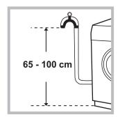
Connect the drain hose, without bending it, to a draining duct or a wall drain situated between 65 and 100 cm from the floor:
