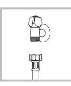
1. Connect the supply pipe by screwing it to a cold water tap using a <sup>3</sup>/<sub>4</sub> gas threaded connection (see figure).
