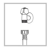
1. Connect the supply pipe by screwing it to a cold water tab using a ¾ gas threaded connection (see figure). Before performing the
