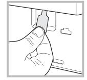
4. pull outwards using the tab as indicated in the figure, until the plastic tie-rod is freed from its stop position; pull downwards and open the door at the same time.
