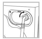
2. Connect the other end of the water inlet hose to the washing machine, screwing it onto the appliance's cold water inlet, situated on the top righthand side on the rear of the appliance (see figure).
