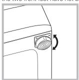
1. Install the washing machine on a flat sturdy floor, without resting it up against walls, furniture cabinets or other. 2. If the floor is not perfectly level, compensate for any unevenness by tightening or loosening the adjustable front feet (see figure); the angle of inclination, measured according to the worktop, must not exceed 2°.
