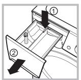
To remove the drawer, press lever (1) and pull the drawer outwards (2) (see figure). Wash it under running water; this procedure should be repeated fre-
