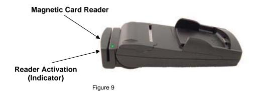
The magnetic read head faces towards the PDA cradle. When placing the card into the reader, the magnetic strip must be facing away from the PDA's cradle as show in the figure below. Keep the edge of the card flat on the inner base of the reader to ensure that the magnetic strip passes over the read head evenly.
