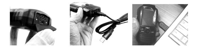
With the computer or power source turned on, the handheld unit will charge its battery over the USB cable. Note: Depending on the model of your computer or laptop used, you may or may not need to power the computer to charge the unit's battery. With power on the cable, the GPS unit will indicate that the battery is charging by way of a message on the unit's screen.
