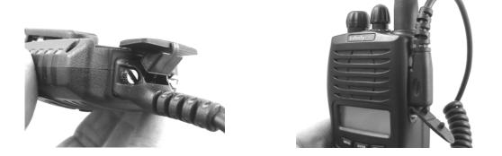
Secure the GPS-MIC-1 cable to the handheld GPS unit using the two set screws provided with the cable. The connection to the GPS-MIC-1 must be flush and level.
