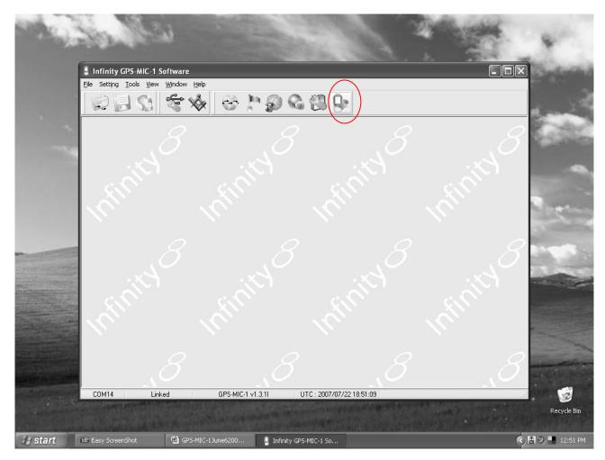
14.3 Once the GPS MIC is linked you will notice the icons on the top right hand side of the program illuminate. Highlight the one that is called firmware tool and click it. The icon is the one on the furthest right.
