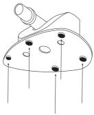
3. Remove the two fixing screws and lift the pivot cover plate off the foot. Use the hex key supplied to loosen the screws.
