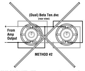
IMPORTANT: When connecting two Beta Ten.dvc subwoofers together, use Method #1 to create a net 4-ohm impedance. NEVER USE METHOD #2, since most amplifiers cannot fully control driver movement in this configuration.
